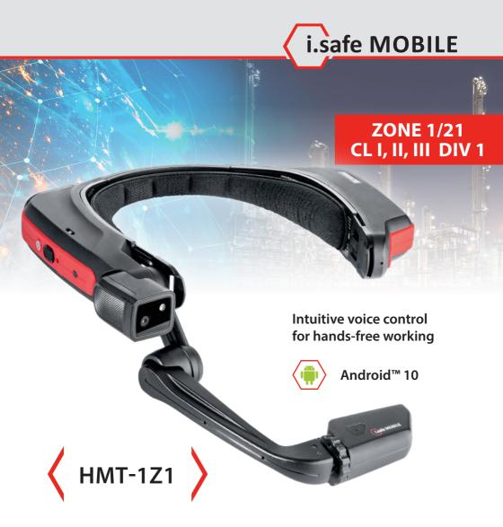
The world's first, voice-controlled tablet for hands-free working in potentially explosive zones 1/21 or CSA Class I, II, III Division 1 is Android-based and has a high-resolution microdisplay. Thanks to its intuitive voice control and digital microphones with active noise suppression, the innovative mobile device is particularly suitable for highly complex remote support applications in noisy industrial environments.
